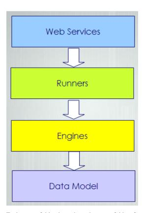
Each source folder depends on the upper folders for compilation. For example, the datamodel is the top level folder so it has no other dependencies on other JABAWS code. The Engine level depends on the datamodel to compile etc. The web services folder is the bottom layer and depends on all the other source code.
