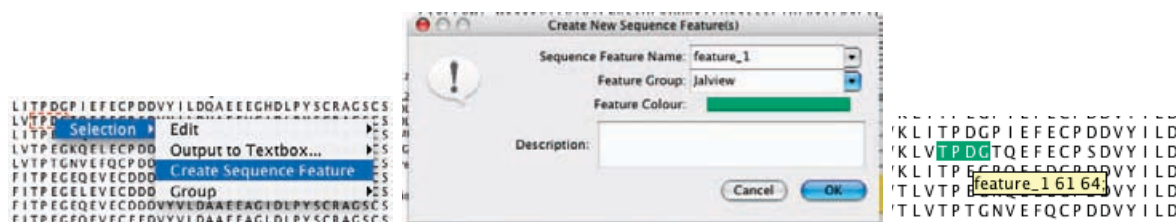
Figure 2.10: Creating sequence features. Features can readily be created from selections via the context menu and are then displayed on the sequence.
